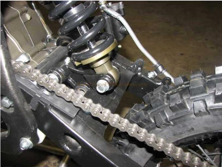
Step 8.) Attach linkage knuckle to swing arm. (Linkage suspension models only. Skip this step if you do not have a linkage suspension model)
