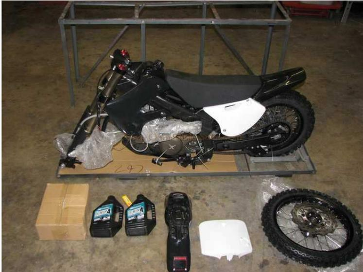
Here is what is inside the small box. Some bike models will have these parts already attached. In this example we are assembling an X5R. The following should be inside the small box: rear shock, right foot peg, bar clamps (3 pieces), gas cap, gas cap breather tube, bar clamp nuts and bolts, top shock mount nut and bolt, bottom shock mount nut and bolt, suspension linkage knuckle bolt, extra spark plug, locktite and extra plastic bolts.
